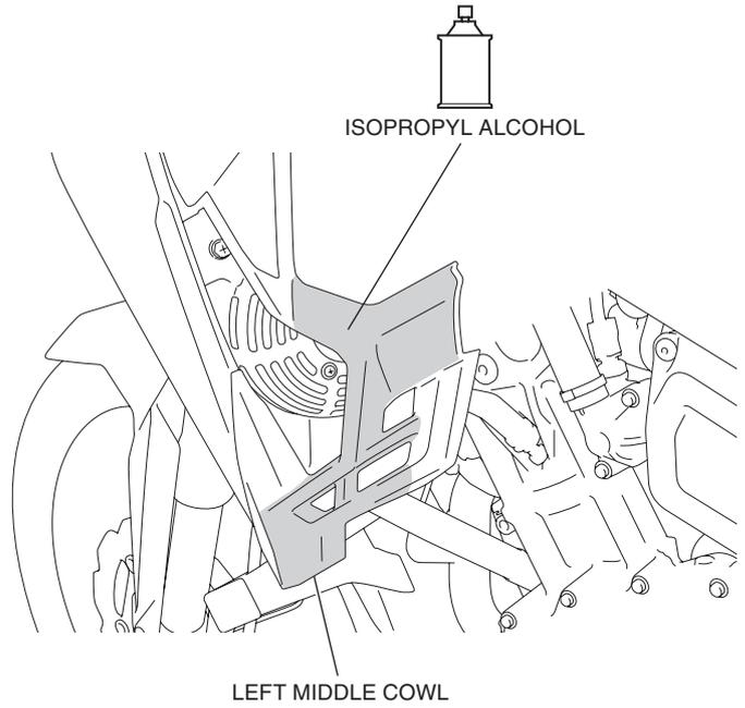
4. Peel off the adhesive backing on the left deflector as shown.
