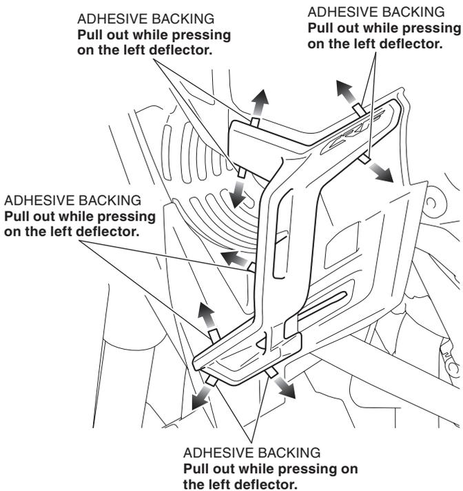
7. Apply adequate pressure to the attached left deflector.
