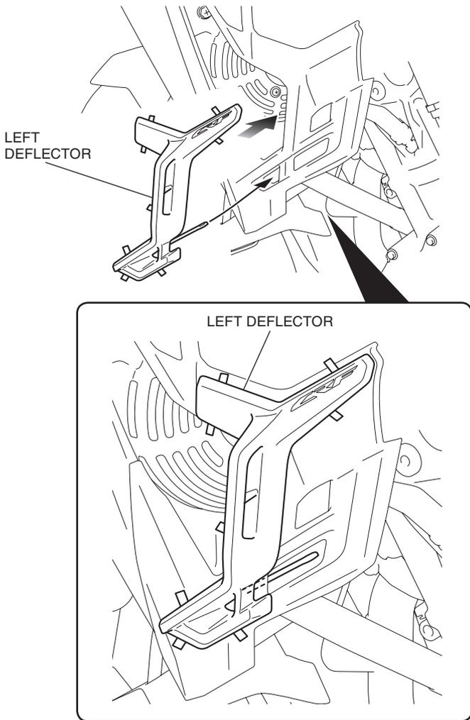
6. Remove the adhesive backing as shown.
