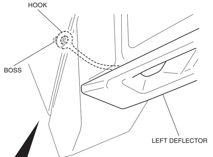
**Install the hook of the left deflector to the boss while expanding the left middle cowl to the outside.**
